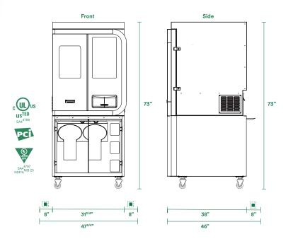
8" Min clearance on all sides | Maximum height measurements. Legs are adjustable
